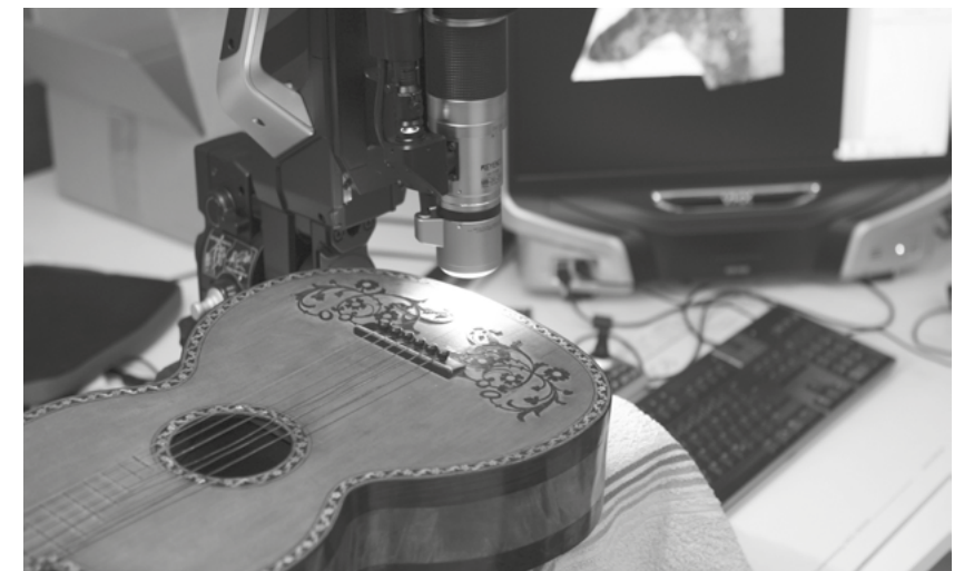
Fig.2 Microscopic investigation of a historical guitar (Beau, build in 1844. MDMB 456) with the digitized image analysis system.
