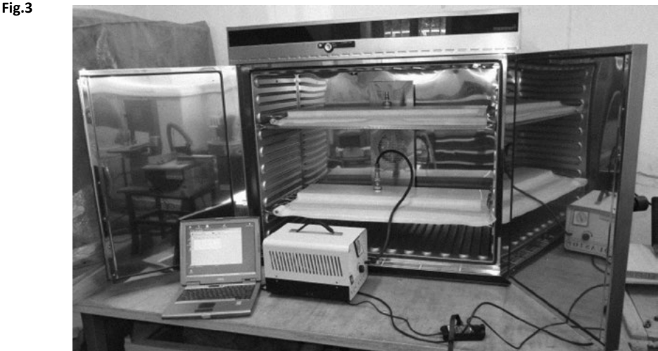
Fig.3 Sealed wood packages in a lab oven during the vaccum procedure.
